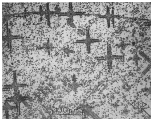
Figure 8 The microstructure on a \{100\} face (on which edge slip bands would normally form) of a pressurized LiF monocystal containing cavities compressed at room temperature 0.6\% at a rate of \sim 2 \times 10^{-4} \text{ sec}^{-1} . The crystal was etched, pressurized at 0.35 \text{ GN m}^{-2} re-etched, deformed and etched again.
